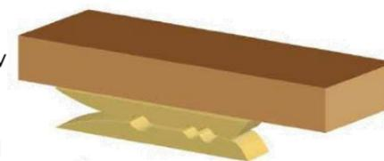
Use **card triangles** with holes for the axle. Check the holes are large enough to allow the axle to move freely. Make sure opposite triangles are aligned carefully so the vehicle moves in a straight line when the wheel and axle mechanism is added.
